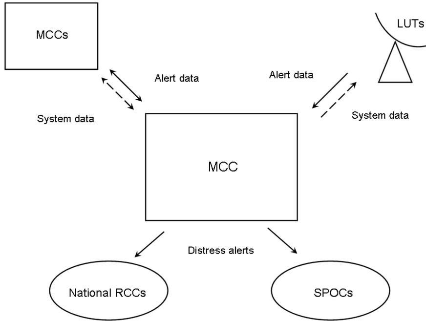
**Figure 2.1: Typical Cospas-Sarsat MCC Functional Block Diagram**
