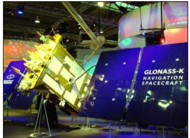
Model of Glonass-K No. 1, the first satellite of the Russian Global Navigation Satellite System carrying a transponder to detect distress-beacon signals.
