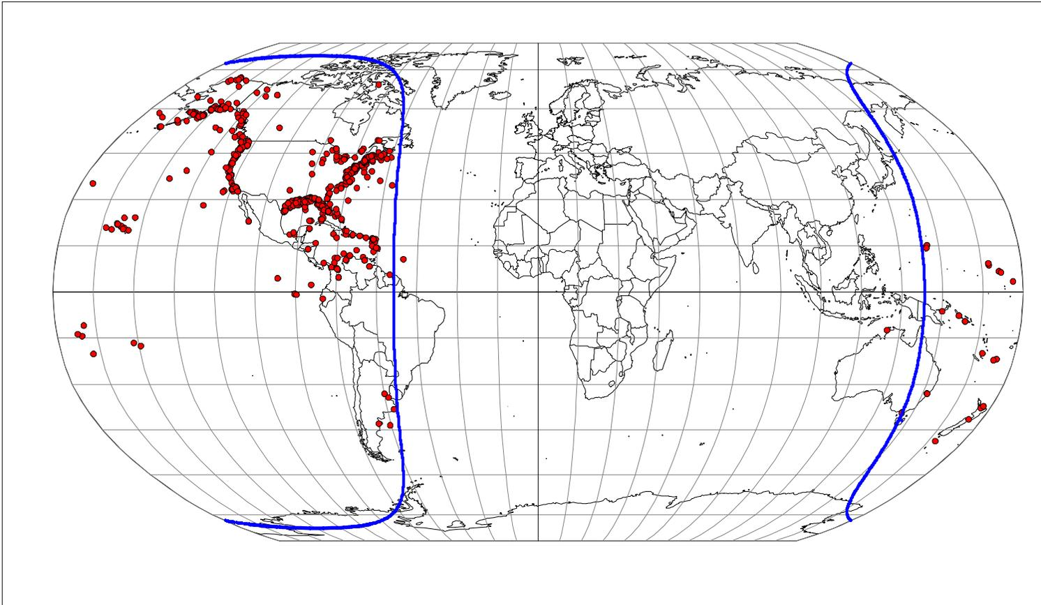
**Figure 4.5: Positions of 406 MHz GEOSAR Alerts as Confirmed by LEOSAR in INSAT-2A Footprint**
