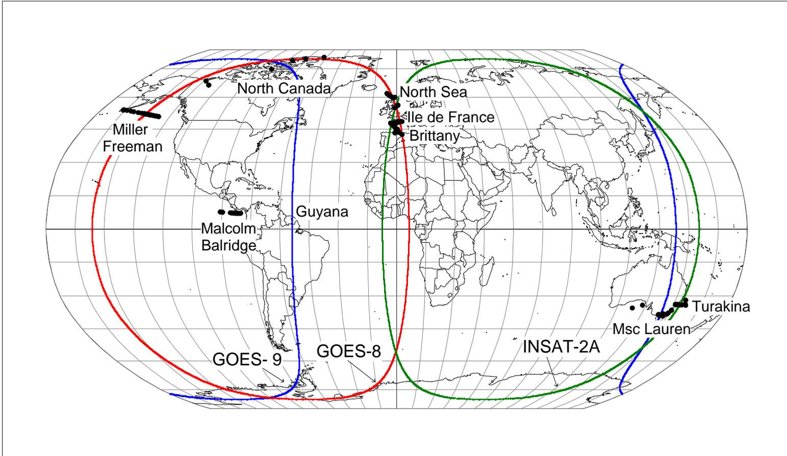
**Figure 3.2: Ile de France Expedition Routes, Coverage and Elevation Angles to Satellite GOES-8**
